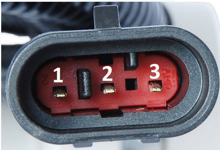
Picture 7. EFLS-A connector terminals location view.
